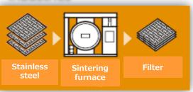
High strength · Heat resistance · Oxidization resistance
